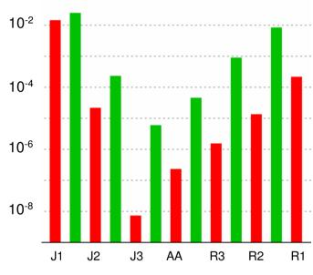
red bars: pressure / [mbar] in respective stages green bars: gas flow / [mbar\*ltr/s] between stages
