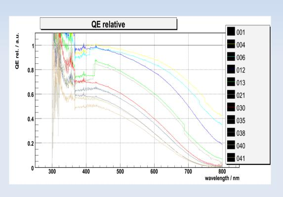
QE drops significantly faster for higher wavelengths
