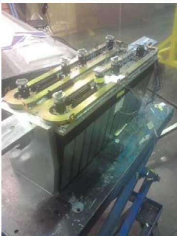
Steel dummy crystals, cooling and support feet
