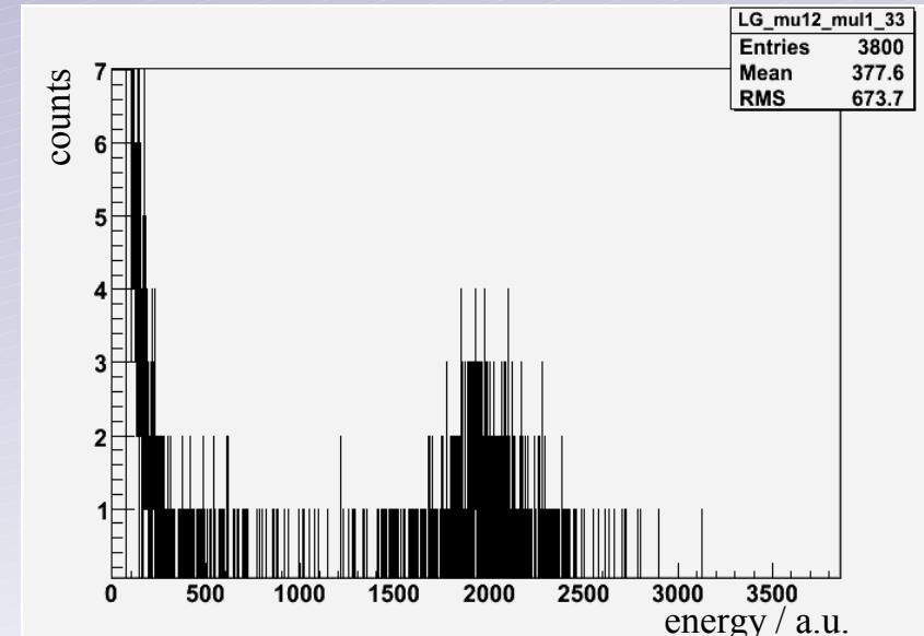
Readout rate about 5Hz → plastic-detectors are not working properly
