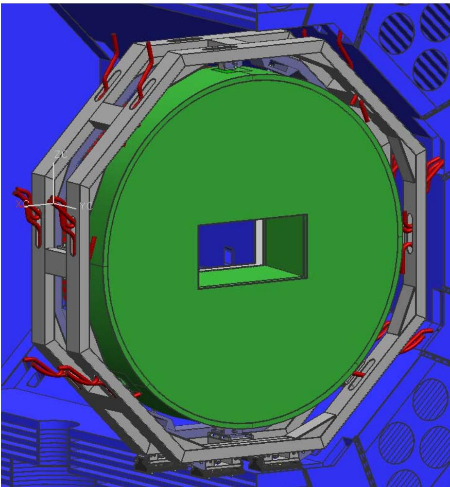
space for cables in hollow frame structure
