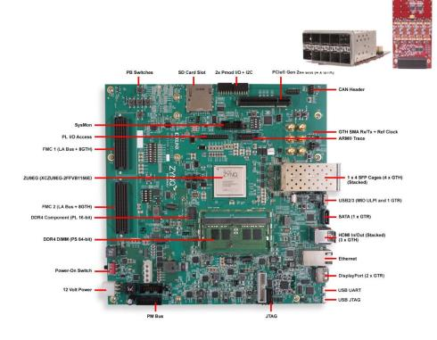
ZCU102 Zynq Ultrascale+ MPSoC XCZU9EG-2FFVB1156 4GB DDR4 20 SFP+ links
