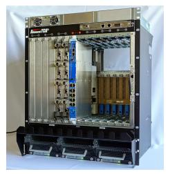
Two fully equipped Compute Nodes, one backplane GbE switch
