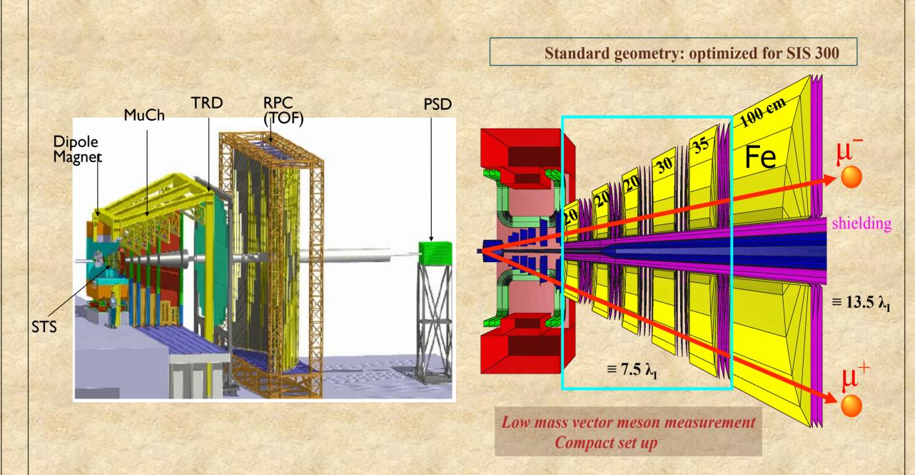
Schematic view of the CBM experiment: Muon set up (left). Implementation of the muon detection system in GEANT (right).
