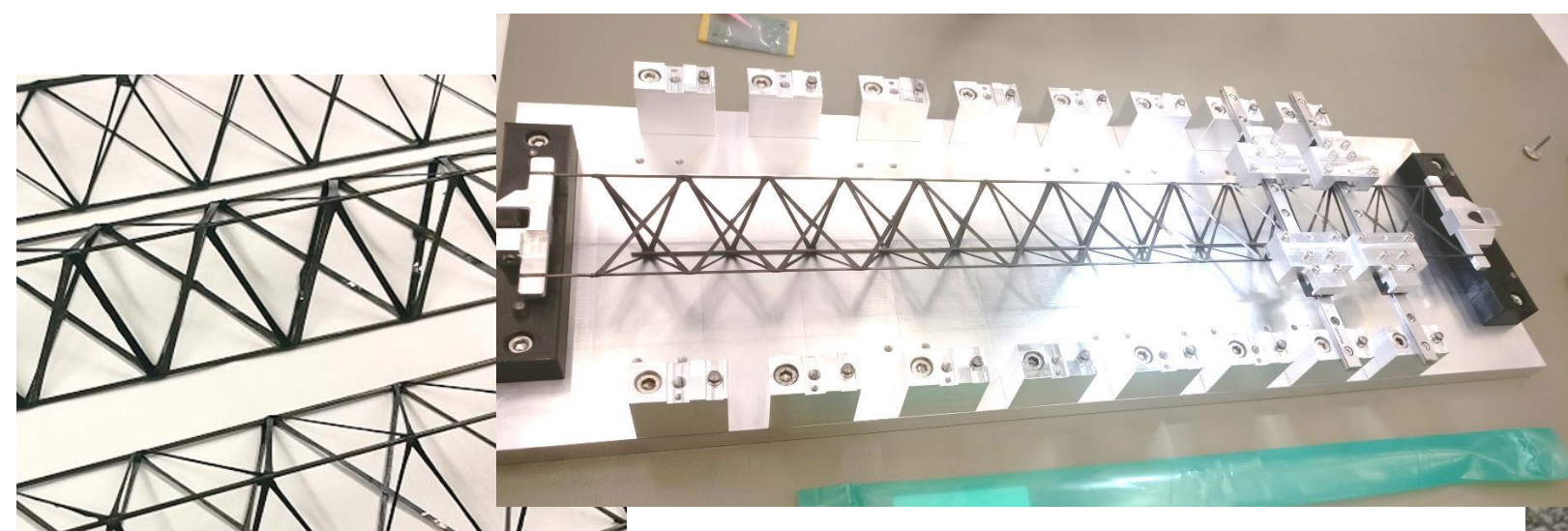
mounting of modules onto low-mass carbon-fiber supports
