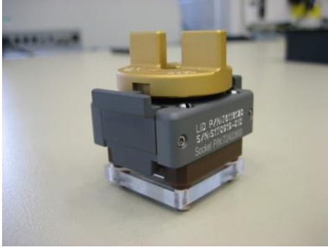
(1) ASIC-test in socket (Pogo pins)
