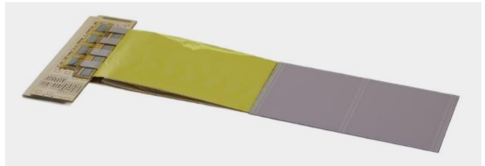
(5) glueing of shielding layers and spacers (6) repeat for reverse module side
