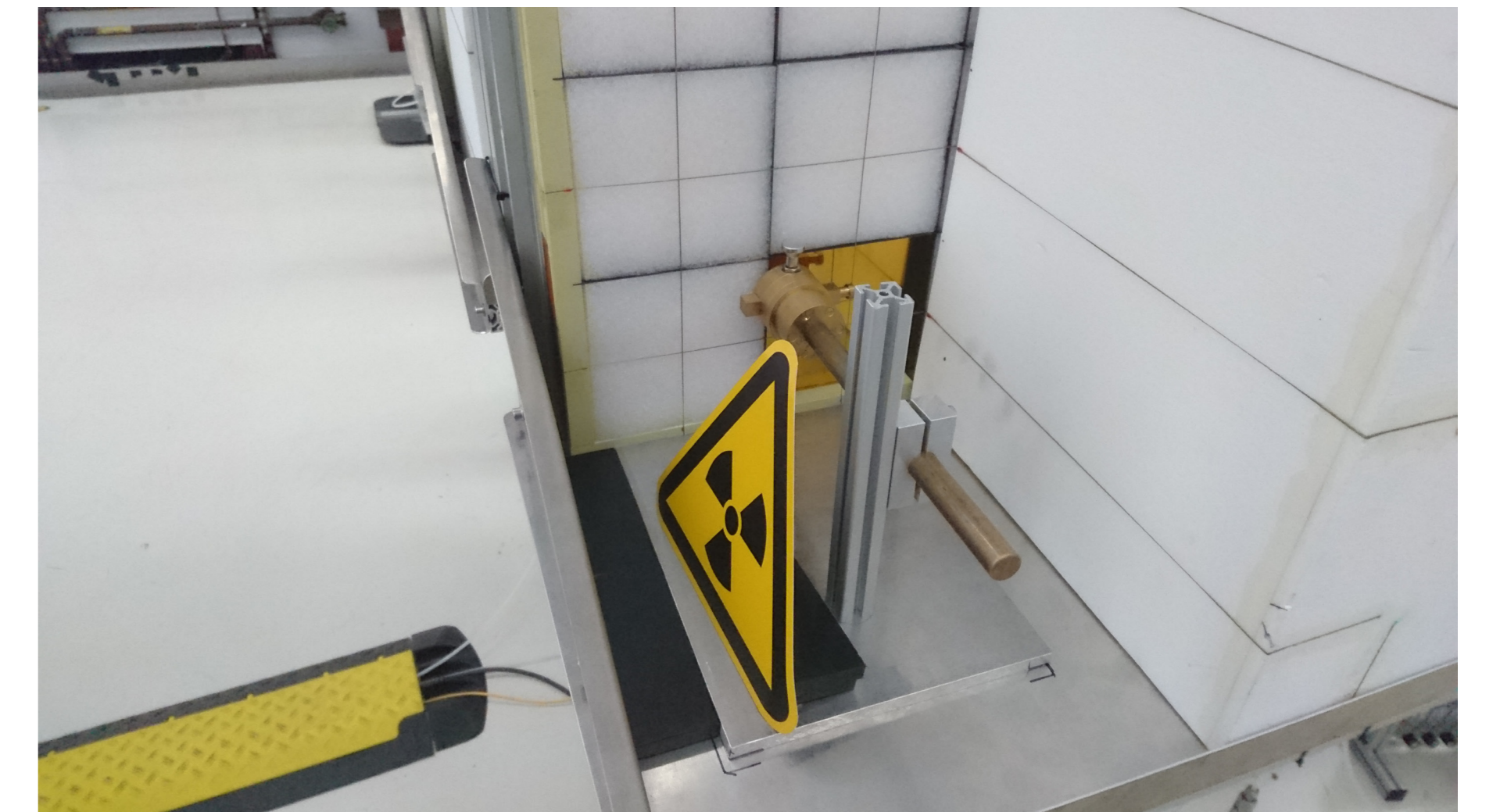
Fig. 3: Positioning of the ^{55}\text{Fe} -source in front of the detector. The golden entrance-window-foil of the MWPC is visible, because radiators were removed in front of the source.
