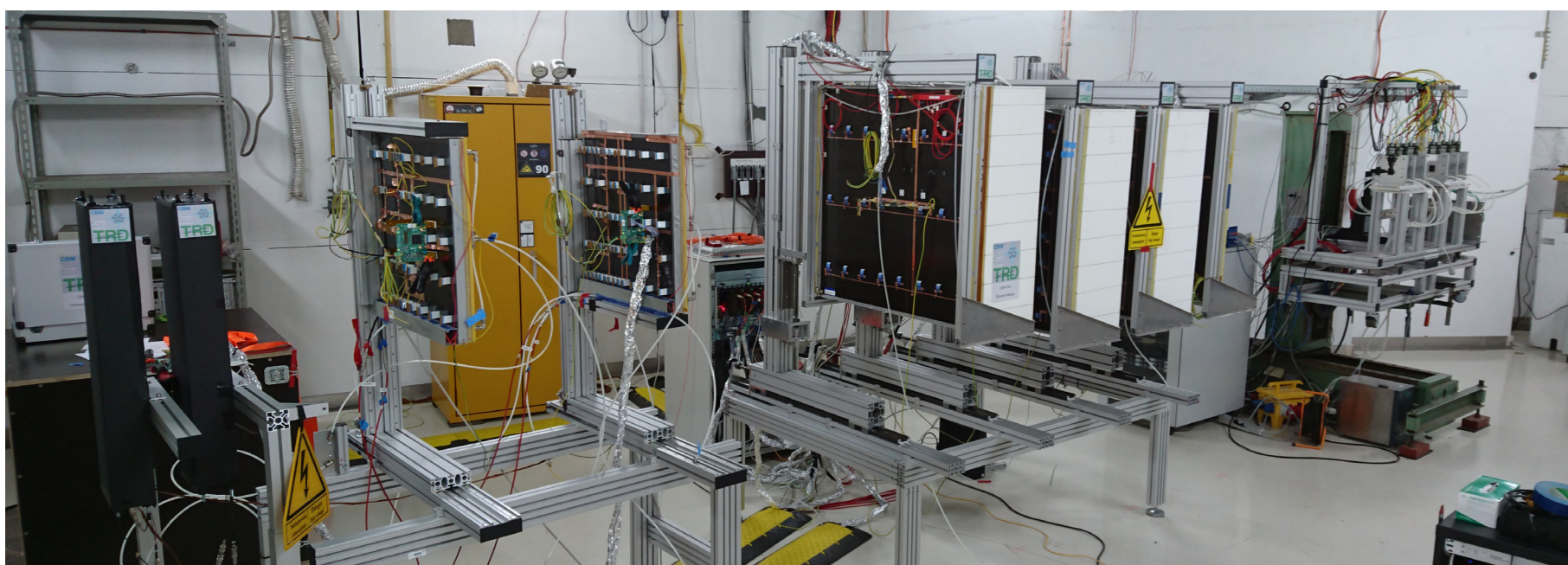
Fig. 1: Setup at DESY T22 in September 2017. From left to right: Two PMT's, two small TRD chambers, one big TRD chamber rotated by 90° with radiator, three big TRD chambers with radiator. Beam from the right.
