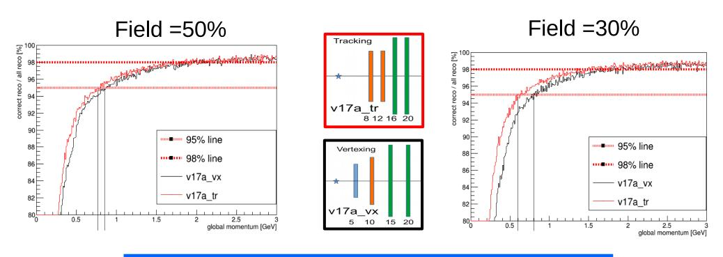
Tracking geometry helps in reconstruction low momentum tracks
