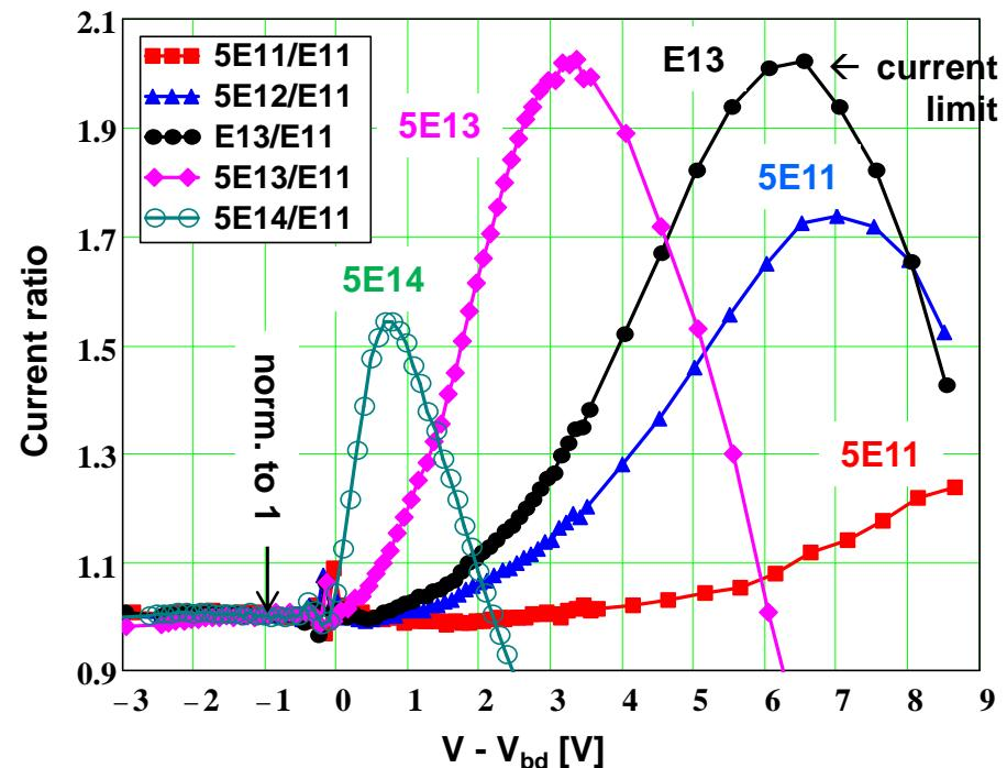
$\rightarrow V < V_{bd} \rightarrow R_{dark} \approx \text{const}; \text{ for } V > V_{bd} \text{ increase by factor up to 2 with } V$
