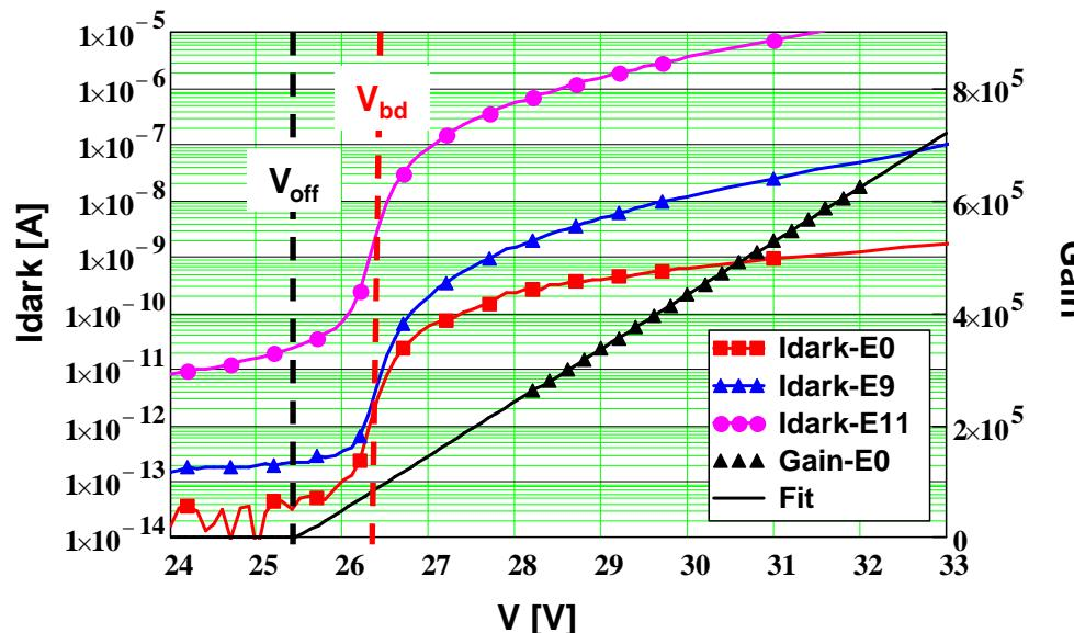
Difference:  $V_{bd} - V_{off} \approx 850 \text{ mV}$  to be taken into account for analysis
