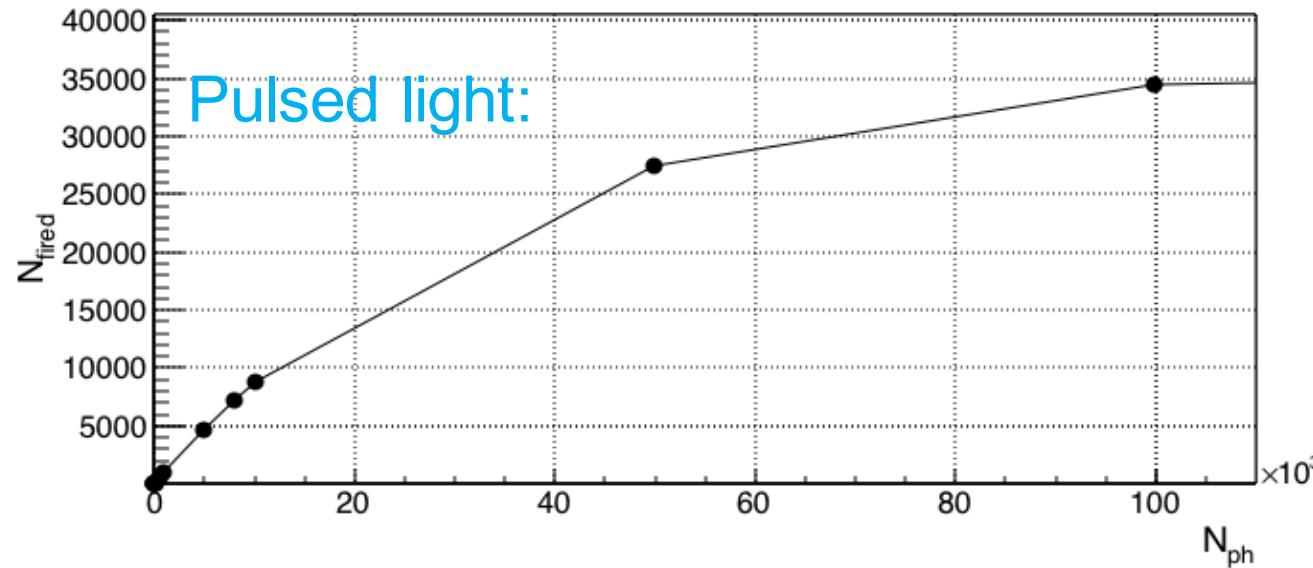
$$N_{fired} = N_{cell} \left(1 - e^{-\varepsilon N_{ph}/N_{cell}}\right) = N_{cell} \left(1 - e^{-N_{pe}/N_{cell}}\right)$$
