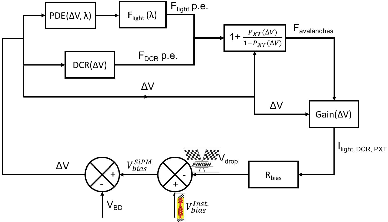
Input parameters:  $V_{BD}$ ,  $C_{\mu cell}$ ,  $R_{bias}$ ,  $DCR(\Delta V)$ ,  $PDE(\Delta V, \lambda)$ ,  $P_{XT}(\Delta V)$
