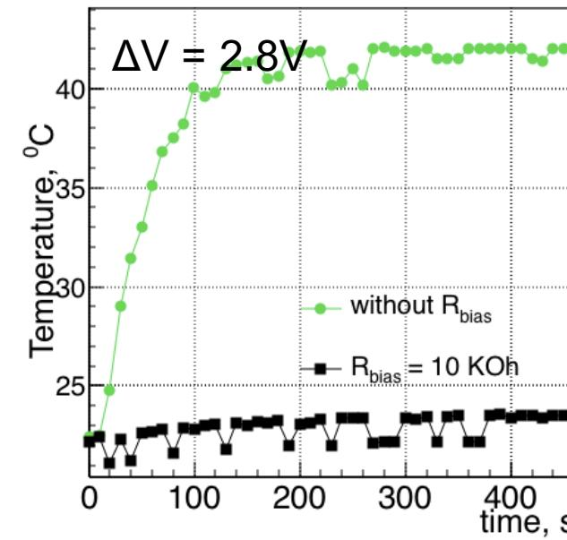
Without  $R_{bias} \Rightarrow$  self heating  $\Rightarrow T^{\uparrow} \Rightarrow \Delta V_{\downarrow}$
