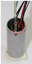
Figure 3.6: Watch out for orientation of aluminum tube. The short GND-strap soldered to the preamp must be joined with the one affixed to the aluminum pipe!
