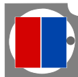
Figure 3.3: Position assignment of BLUE and RED labeled APDs in the capsule (capsule shown from front, looking at the sensitive surface of the APDs).
