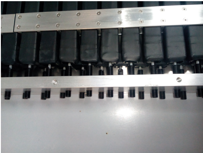
Abbildung: Each bar is pressed against the SiPM via spring loaded pins.
