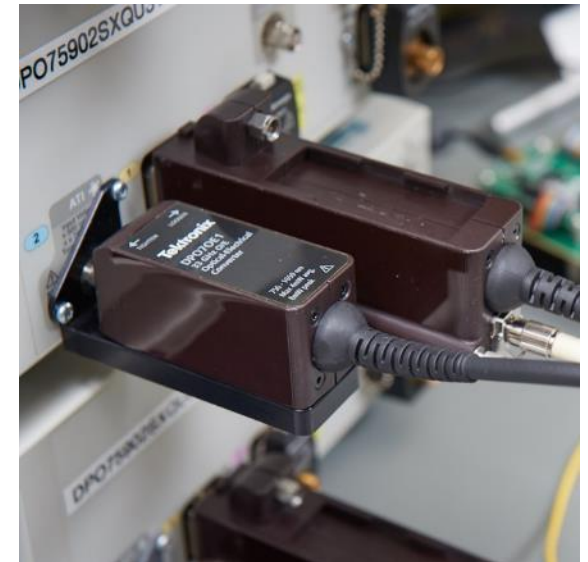
ATI – Mechanical support deck
