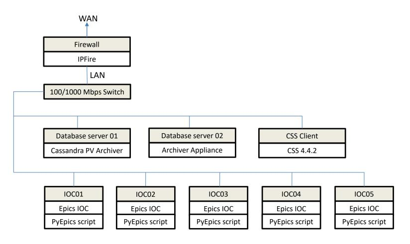
**Db Servers, CSS Client, & IOC01- 03** - 2x Dual-Core AMD Opteron 2216, 8 GB RAM (Dell SC1435) **Firewall, IOC03-04**: Intel Xeon CPU 3.00GHz, 4 GB RAM (Dell SC1425) IOC.... Epics IOC PyEpics script EPICS 3.14.12.7
