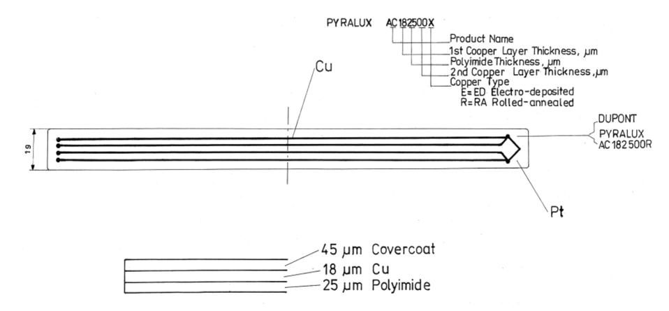
A contact between the Cu lines and the sensor is provided by two circular islands (ca. 1mm in radius) where Pt and Cu layers overlap. The width of Cu lines is also 1mm. The section of the laminate together with the isolating covercoat demonstrates that the overall thickness will not exceed 90 microns.
