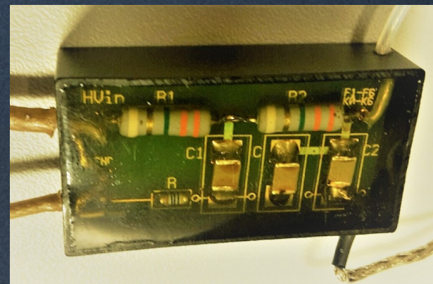
HV filter: resistors 2x 1.1M \Omega
