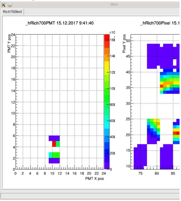
Left histogram shows the mocked up PMT positions in the future RICH700 backplane array, right histogram the pixel positions on such plane (zoomed to the interesting region with our 12 testbeam PMTs)
