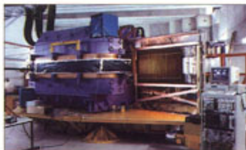
GSI Darmstadt's kaon spectrometer, KAOS, looks at the kaons emerging from heavy-ion collisions. (Photo Achim Zschau/GSI.)
