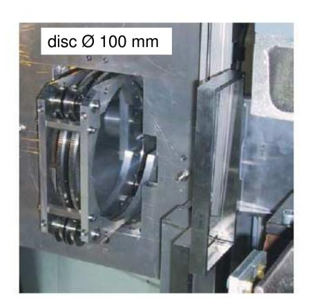
Wedge shaped disc and double-shaped wedge machined with  $\mu m$  precision.
