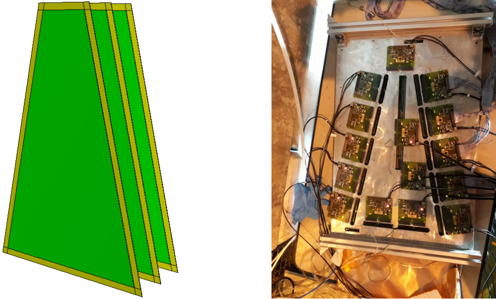
Figure 15: (left panel) - the present CbmRoot geometry of three GEM modules forming the mMUCH subsystem. (right panel) - photograph of a trapezoidal module mounted on a Aluminum plate used during the CERN-SPS test in 2016.
