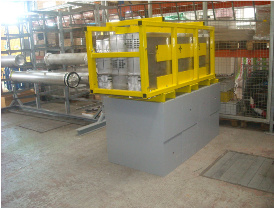
Figure 23: Assembled mPSD supermodule near the test beam line at CERN.
