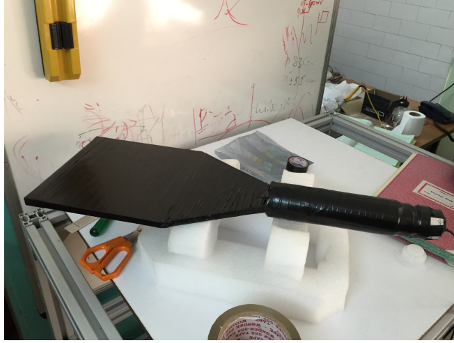
Figure 4.6: Completed scintillator paddle detector
