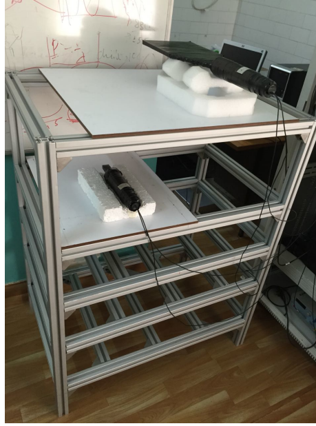
Figure 5.2: Experimental set-up to study angular variation of cosmic ray flux
