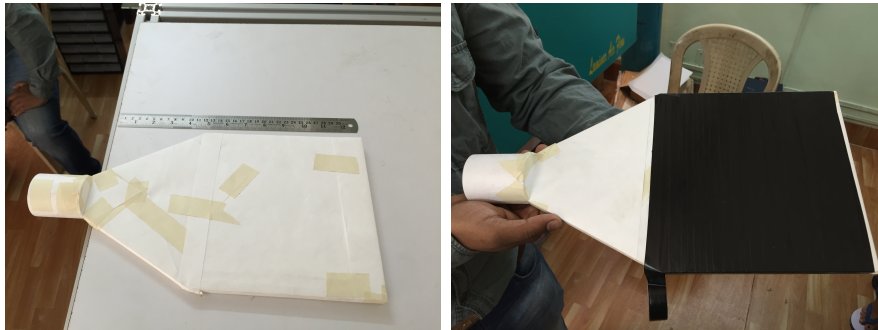
Figure 4.3: Wrapping with Tyvek paper (left) and with black tape (right)
