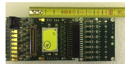
FE-board with ASIC
