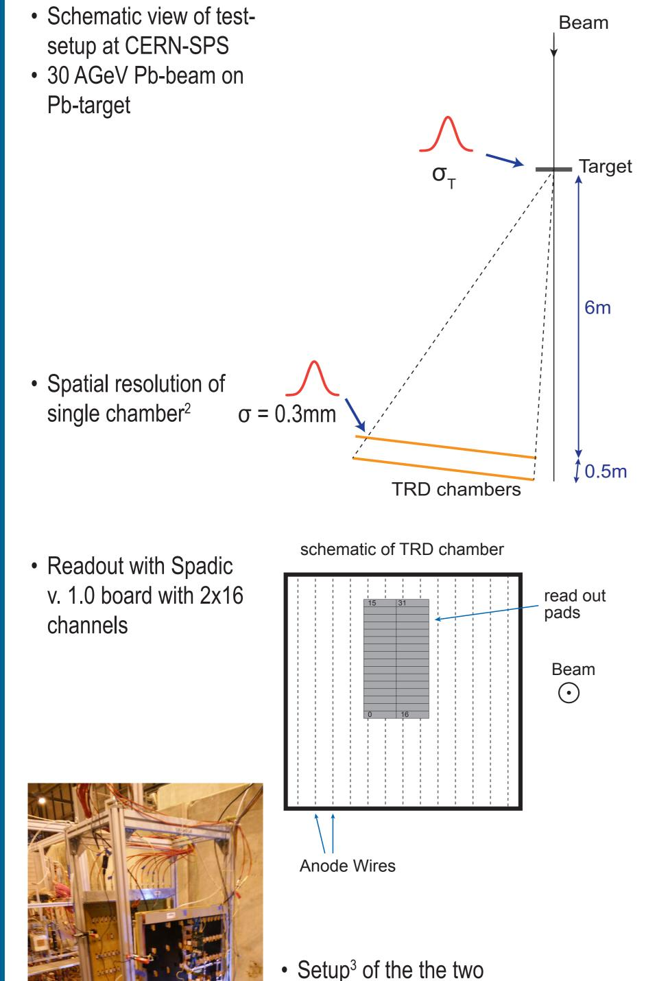
We analyze the **common spatial resolution** of the TRD-prototypes by looking at hits occurring in the same time-slice on both chambers.
