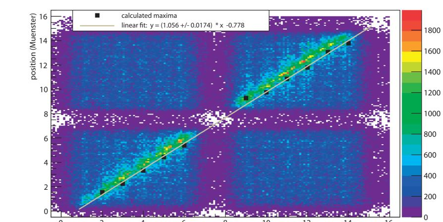
The small tilt in the maxima of hit coincidences is a result of the geometry of the test setup. This needs to be corrected. In order to do this, we need to find the linear correlation, formed by the maxima in the histogram. Position is given as pad-number.
