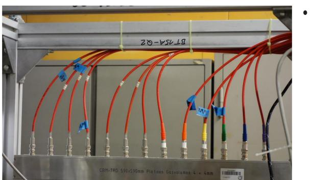
Connection of HV Supply to 13 segments of TRD
