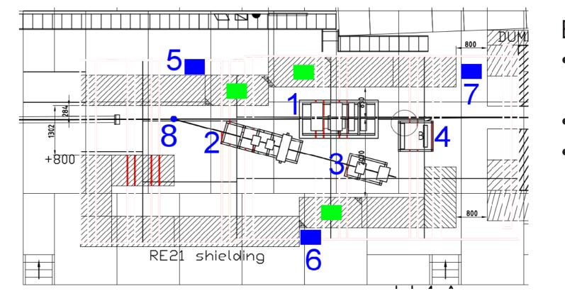
Blueprint<sup>1</sup> of setup in cave TRD prototypes from IKF and IKP at pos. 4 • HV supply at pos. 7 • Target at pos. 8
