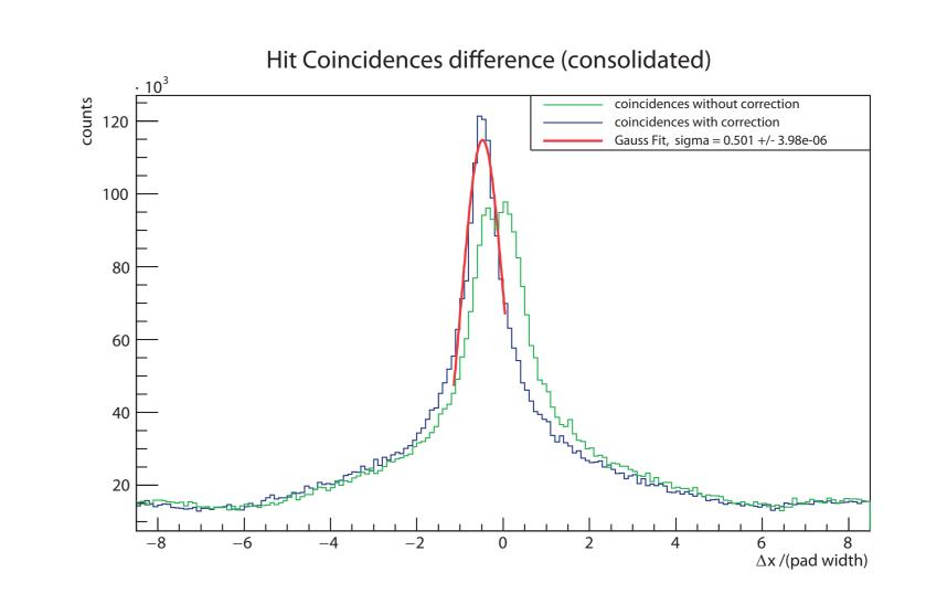
After correcting and plotting the difference of hit positions, we can calculate the spatial resolution by performing a Gaussianfit. With a pad width of 7mm, this results in:
