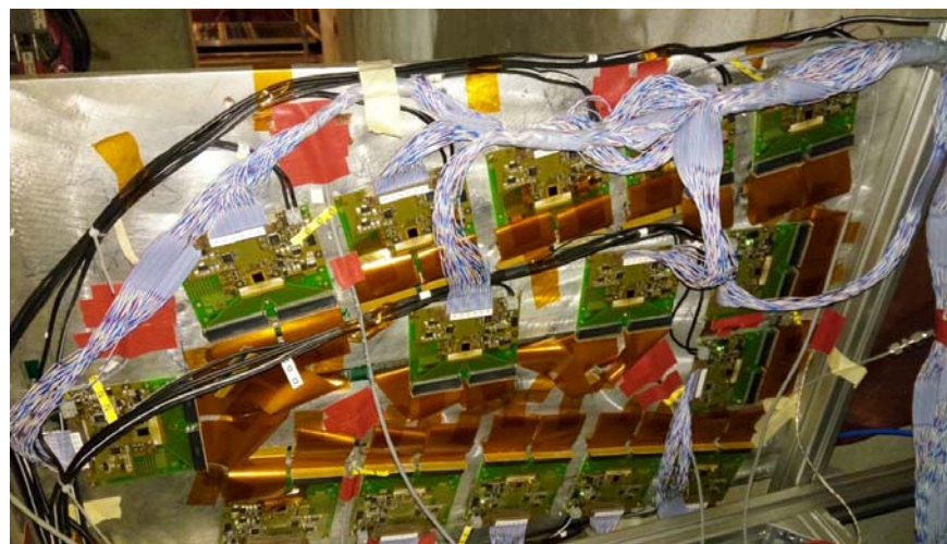
Full size GEM detectors tested with free-streaming read-out electronics at the CERN-SPS Nov.-Dec. 2016
