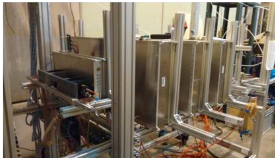
ToF MRPC detectors tested with free-streaming read-out electronics at the CERN-SPS Nov.-Dec. 2016
