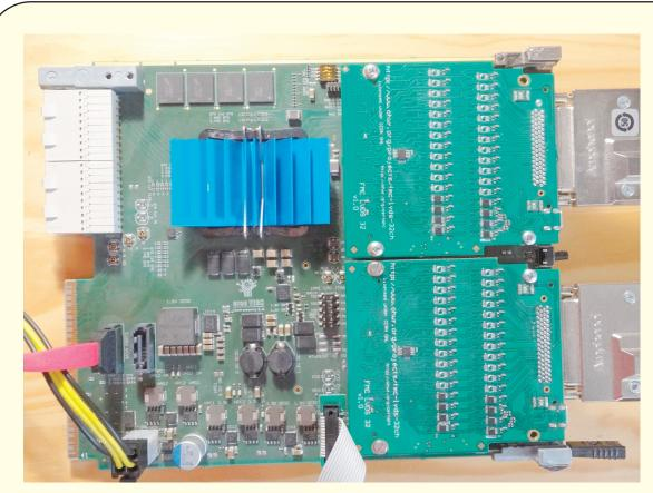
AFCK board with two connected FMC/VHDCI boards. The differential link is provided by the VHDCI cable.
