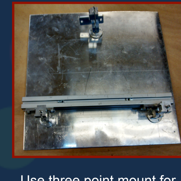
Use three point mount for mirror tiles in order to reduce material budget
