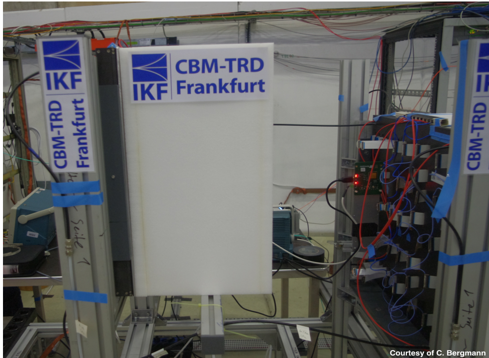
Figure 8.4: The two Frankfurt TRD prototypes used in the CERN-PS test-beam in 2014. A polyethylene foam foil radiator was used for both Frankfurt prototypes.
