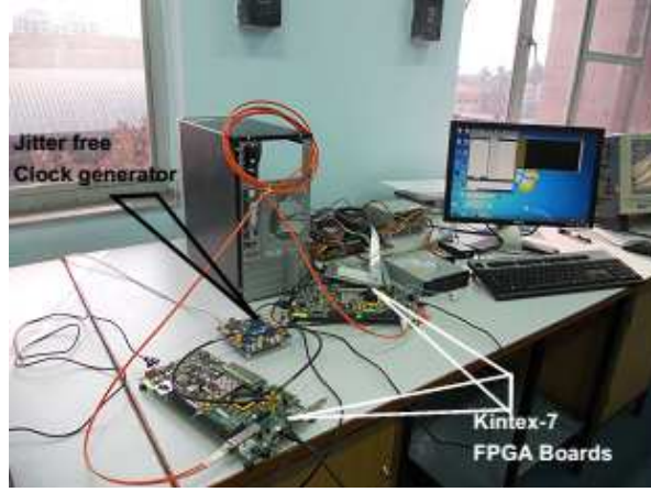
Figure 4.20: System for testing the proposed DAQ system using KC705 and external clock generator
