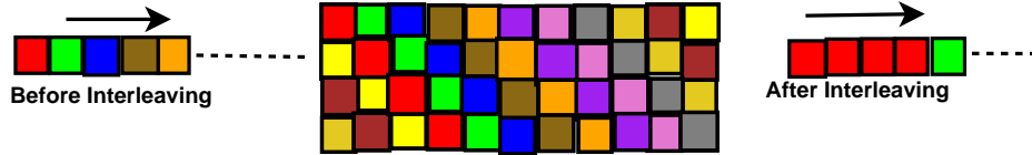
Figure 4.8: Helical Interleaving Process
