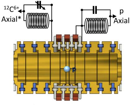
\*Resonator fine tuned with a varactor diode
