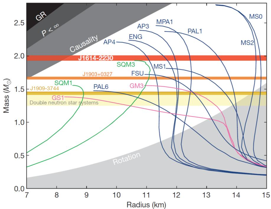
Soft EOS (Skyrme,  $K = 200$  MeV) is not repulsive enough to allow for a neutron star with 2 solar masses.
