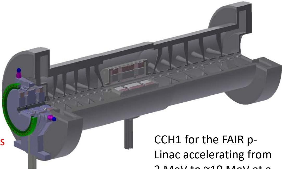
CCH1 for the FAIR p-Linac accelerating from 3 MeV to ~10 MeV at a length of 1.5 m.
