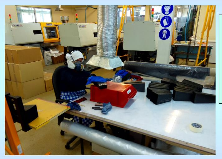
About 1500 single carbon fiber alveoli units have to be prepared for gluing in packs.
