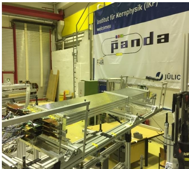
Straw test system and front-end electronics.
