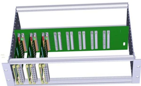
HV crate for tests with HV decoupling boards and additional amp board.
