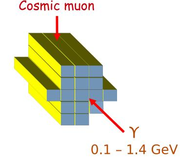
16 PbWO<sub>4</sub> crystals + LAAPD + Basel LNP Pre amp + SADC (100 MHz, 16 bit)
