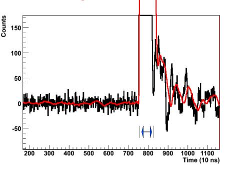
Afterpulses are exceeding 1 MeV for large energy deposits ~ 1 GeV, contribute 0.5% of the main pulse and are excluded by time window
