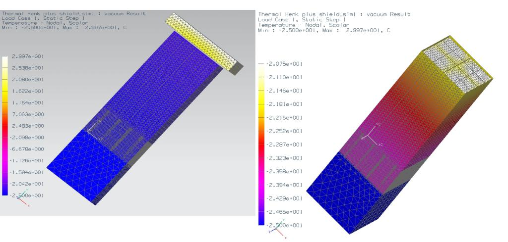
even with vacuum insulation: temperature gradient of 4 K
