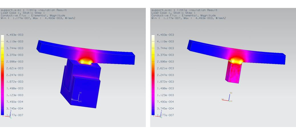
work in progress, preliminary resultson heat flux: max. 5 mW /mm<sup>2</sup> seems acceptable
