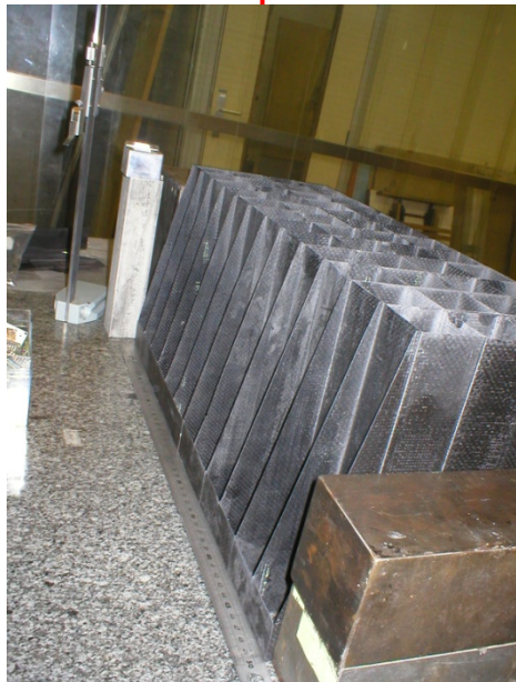
Gluing of 240 carbon alveoles
