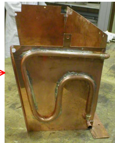
Side Cooling System
