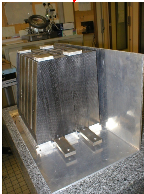
Gluing of 240 Stainless Steel Crystals
