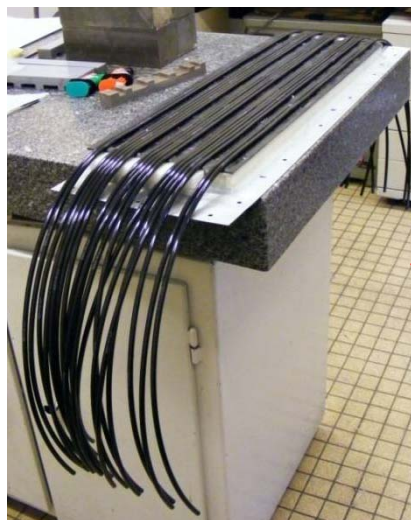
Lower Cooling System (Vacuum system)
