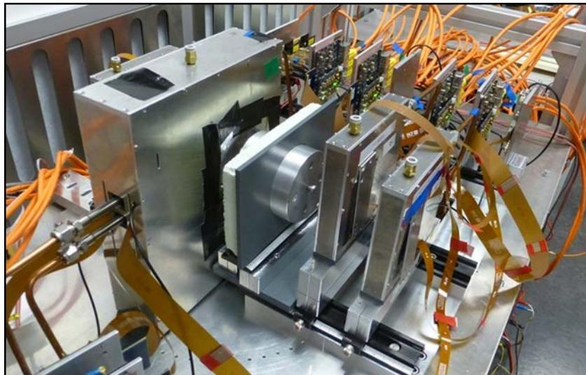
The MVD consists of highly granulated Monolithic Active Pixel Sensors (MAPS) arranged in four ultra-thin detector arrays positioned close to the target. Determination of secondary vertices with high precision which is required for the identification of charmed mesons.
