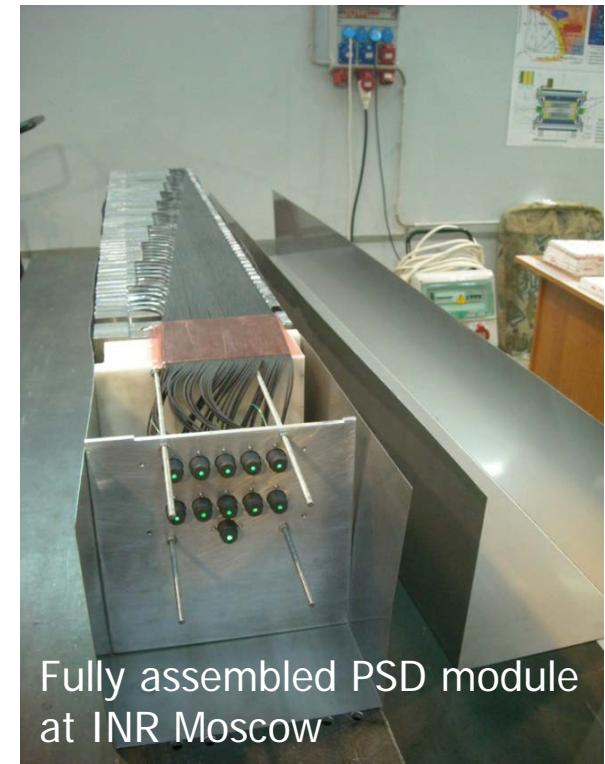
The PSD is a lead-scintillator calorimeter and is used for the determination of the collision centrality and the orientation of the reaction plane.
