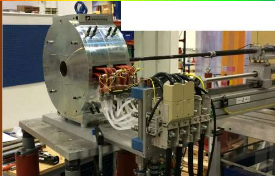
SOLENOID B Module 2 Factory Acceptance Test
