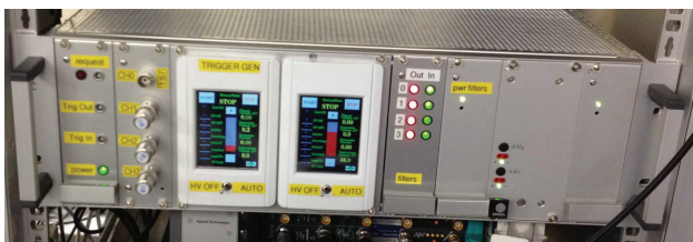
Figure 1: Two units for control of HV generators of UEWE dynamic target for PRIOR.
