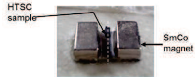
Fig.6. HTSC sample aligns inside the PMG with the line of minimal magnetic induction. The HTSC samples have been made at LPI from \text{YBa}_2\text{Cu}_3\text{O} ceramics ( T_c \sim 91 K, H_c \sim 5.7 T at 0 K)
