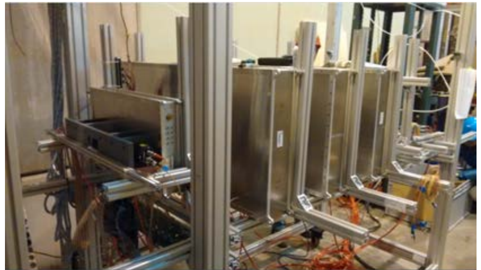
ToF MRPC detectors tested with free-streaming read-out electronics at the CERN-SPS Nov.-Dec. 2016
