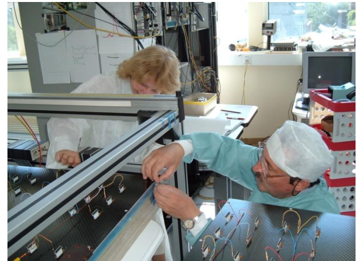
Final tests: gain uniformity & energy resolution @ 55 Fe source
