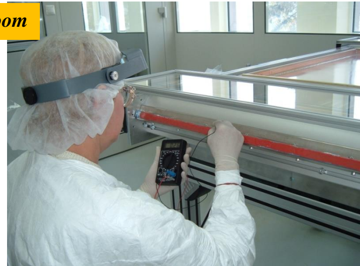
Final tests: gain uniformity & energy resolution @ 55 Fe source
