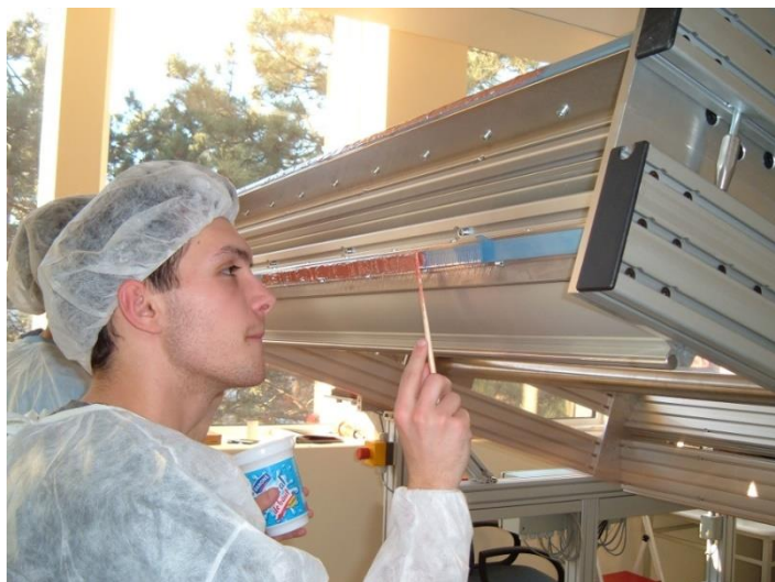
Multiwire electrodes winding using winding machine
