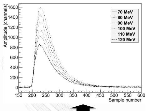
Proton traces from the Flash ADC de-noised using a wavelet decomposition and filter procedure
