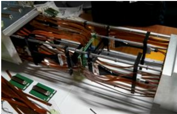
Active Si stopper used at RIKEN, where 2-mm thick 65 x 45 mm 2 plastic detectors were sandwiching 5 Si DSSSDs, with an estimated efficiency of 30%. On the right hand side a sketch of the implantation segmented fast plastic is shown.
