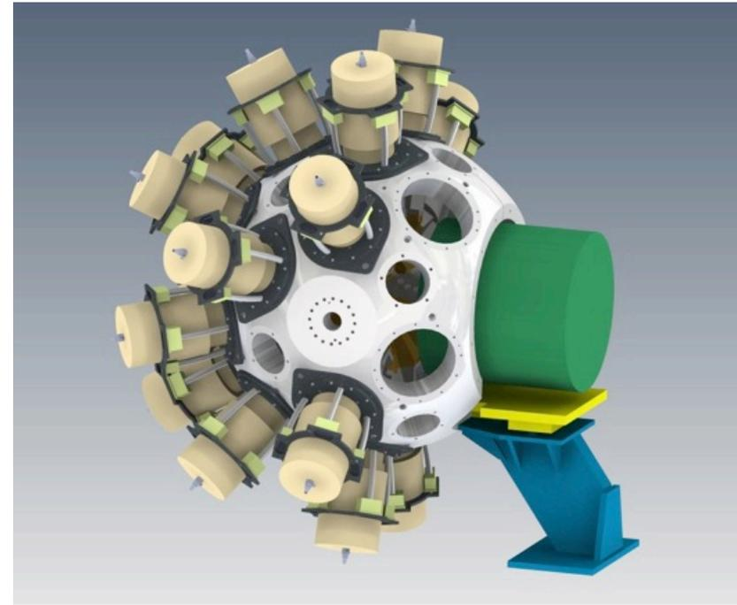
Will fit inside GRETINA frame (most forward detector ring removed)
