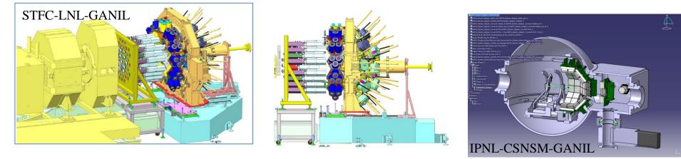
The final mechanical design of NEDA + NWALL foresees the use of 54 self produced NEDA detectors at forward angles and 14 NWALL detectors at around 90 degrees
