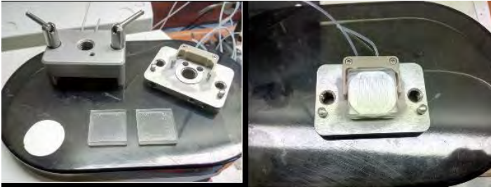
PHASE SEPARATOR (PTFE OR PVDF HYDROPHOBIC/HYDROPHILIC MEMBRANE + UNDERPRESSURE)
