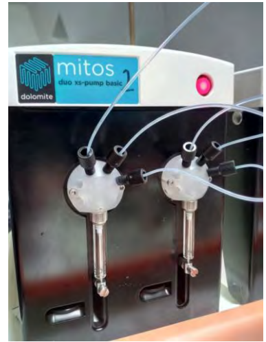
SYRINGE PUMP (6-CHANNEL VALVE, VOLUME ADJUSTABLE BOTH BY SYRINGE AND SOFTWARE)
