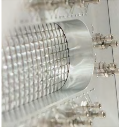
RTC window supported by piano wire, In SISAK LBNL experiment in 2000.
